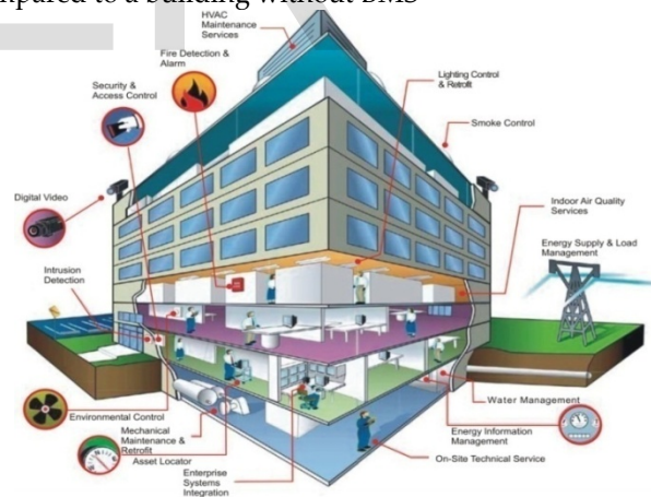
Figure: 10 A fully optimized BMS system
